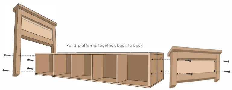
Use 2 or 2.25 inch screws to attatch headboard legs. Screw from the back of the legs into the storage frame.
